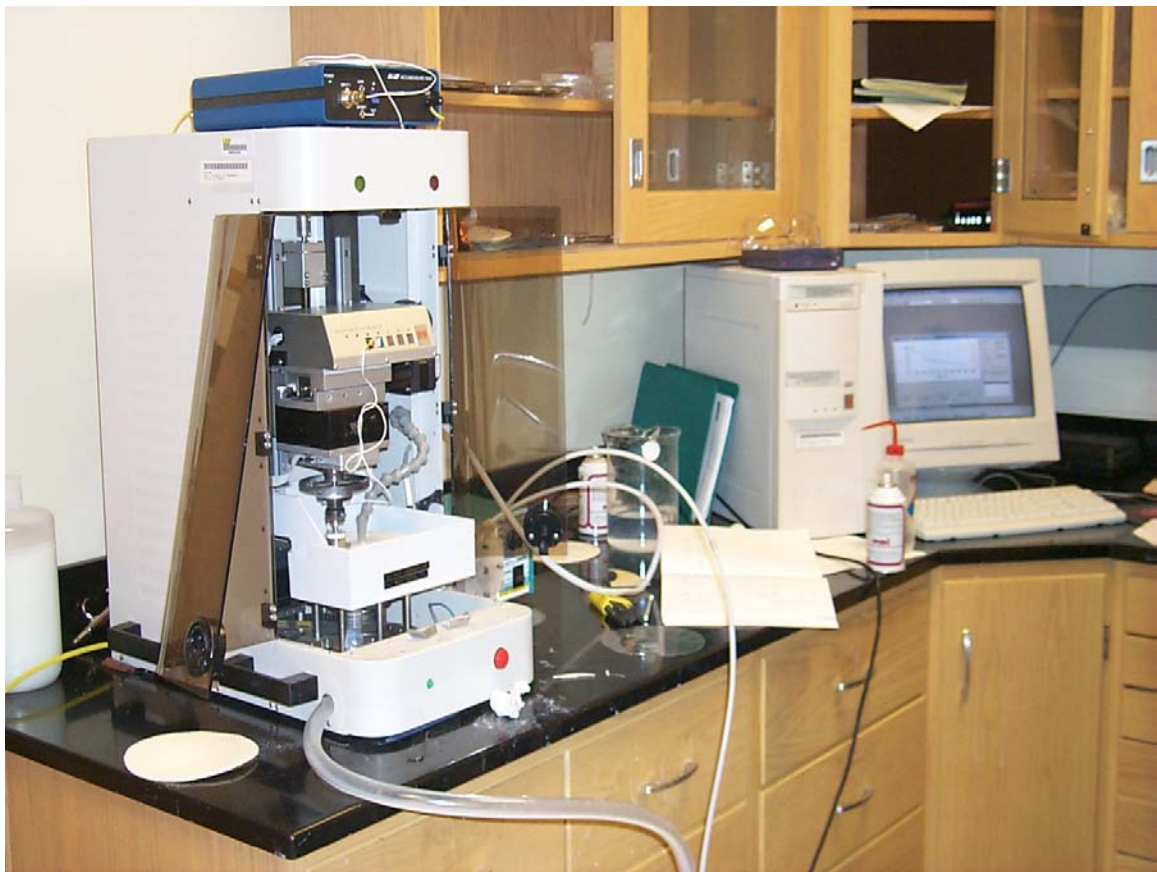
Figure 6 Universal micro tribometer with PC based feed back control
