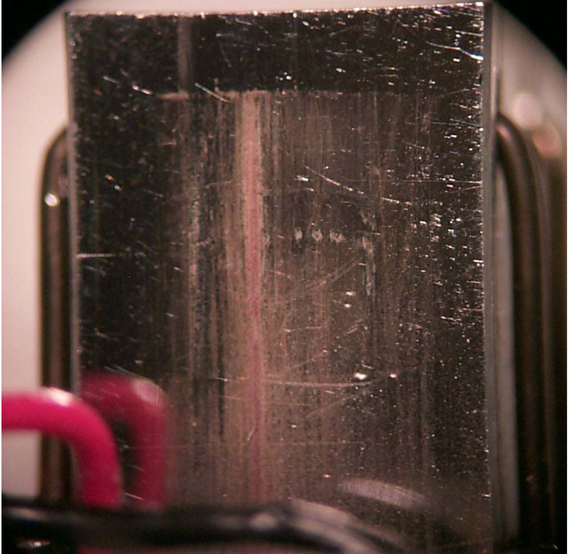
Figure 20 Motor prototype part surface nearest actuators after 1.243mile (2km) sliding endurance test (made of 52100 steel gage block)
